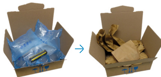
EXAMPLE OF PACKAGING OPTIMIZATION: REDUCTION OF PLASTIC PACKAGING BY SWITCHING TO CARDBOARD AS FILLING MATERIAL (PILOT PROJECT IS STILL IN THE IMPLEMENTATION PHASE)
