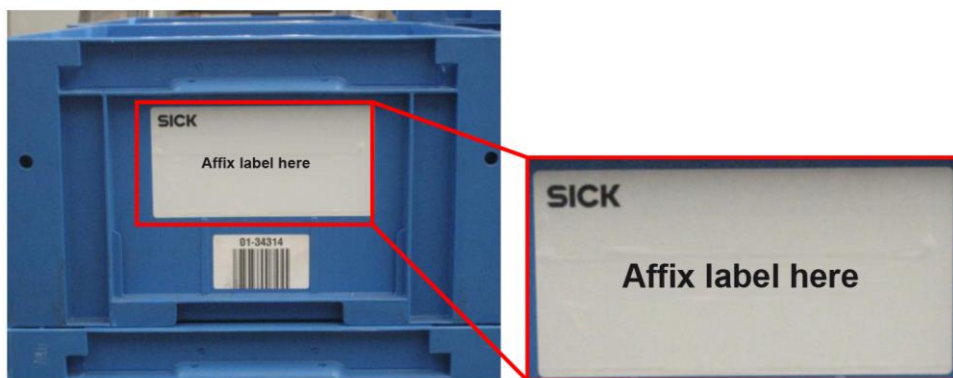
Figure 1: (left) container with so-called landing place label. (right) landing place label; labels / container labeling must be affixed here
