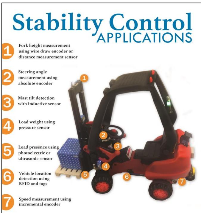
The most common types of sensors detect the following:
