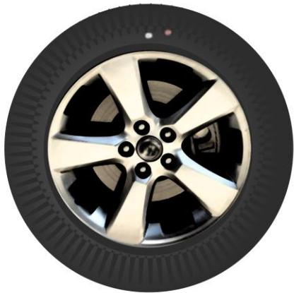
Just as perfect roundness is never wholly achievable, perfect balance between the tire and wheel is also extremely difficult to come by. By mounting a tire so that its light balance point is aligned with the wheel's heavy balance point, the amount of weight needed to balance a tire and wheel assembly is minimized. Therefore, tires are marked with yellow dots at their light balance point. (Generally, the heavy balance point of a wheel is at the valve stem.)
