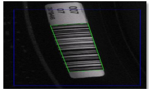
Laser-based bar code readers, used for years to track and sort tires throughout the production process, have long been the de facto standard for track and trace in the industry. However, historically marker dots were either inspected manually or not at all. This situation has changed with the strict requirement of dot verification.
