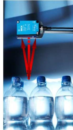
Using two redundant receiver arrays, this sensor is able to detect shiny, glossy or dark targets within its foreground without signal interruptions by reliably capturing the redirected light, regardless of the target's reflectivity characteristics.
