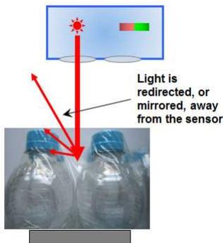
Similar problems also frequently occur with dark or low-remission targets such as clear shrink wrap, which may not return sufficient light for the receiver array to detect its presence.
