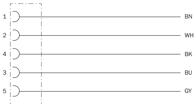
Contact assignment of the M12 female connector
