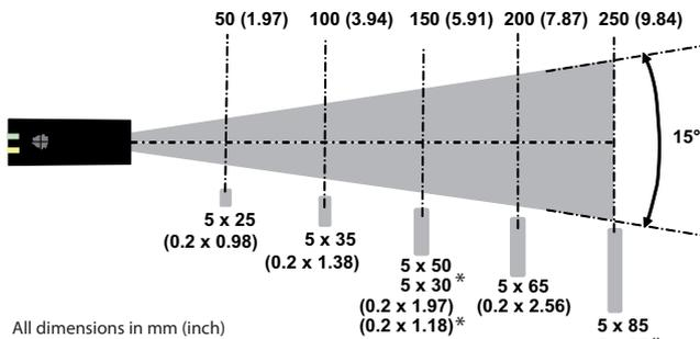
\* The angle of reception is smaller than the angle of dispersion therefore the effective length of the light spot is smaller than the real visible line-shaped light spot.
