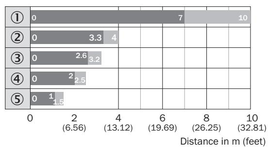
■ Sensing range ■ Sensing range, max. typ.
