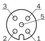
female connector M12, 5-pin, D-coded
