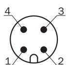
Connector M12, 4-pin, A-coded
