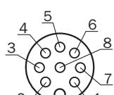
female connector M12, 8-pin, A-coded
