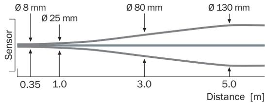
Sensing range diagram GL6, GL6G
