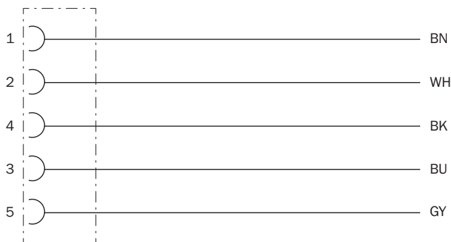
Contact assignment of the M12 female connector
