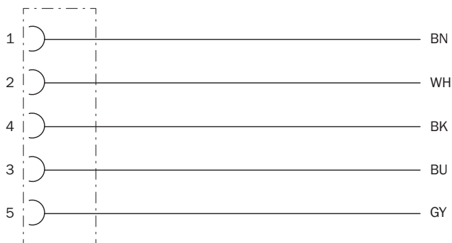
Contact assignment of the M12 female connector
