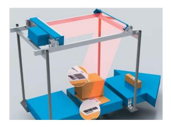
Figure 7: A line scan camera identifies 1D and 2D codes on objects of different heights, which are carried through the camera's reading area by belt.
