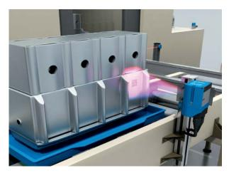
Figure 8: Matrix cameras read printed or directly marked 1D and 2D codes, for example during the package sorting process (left) or for unique identification of parts such as motor blocks during production (right).
