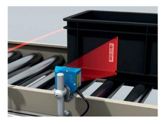
Figure 5: Laser scanners are widely used in warehouses because they securely identify the load carriers when laterally mounted on the conveyor system. The diagram shows a line scanner which is activated by a photoelectric sensor.
