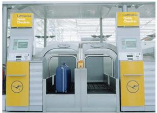
Figure 1: Combinations of the RFID and laser scanner technologies are used, for example, at airports in luggage identification systems for luggage sorting (left) and in self-bag drops (right).
