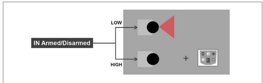
Fig. 59 Switching the laser scanner to sharp/not sharp (switching input Armed/Disarmed)
