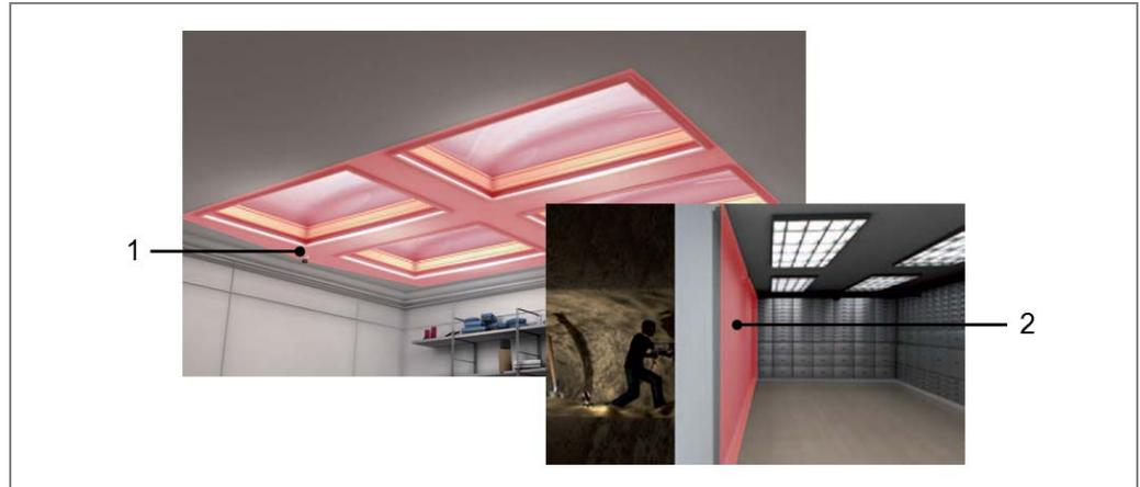
Fig. 18: Ceiling monitoring and wall penetration protection
