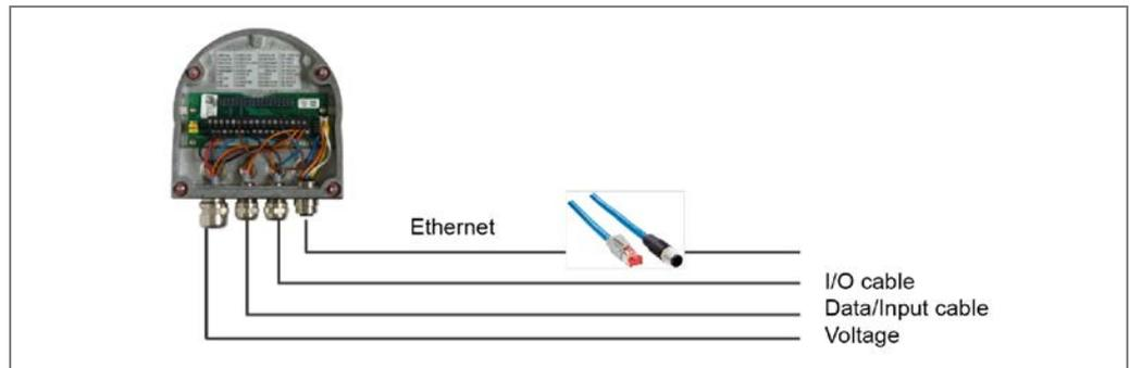
Fig. 24: LMC12x/LMS12x connecting cables
