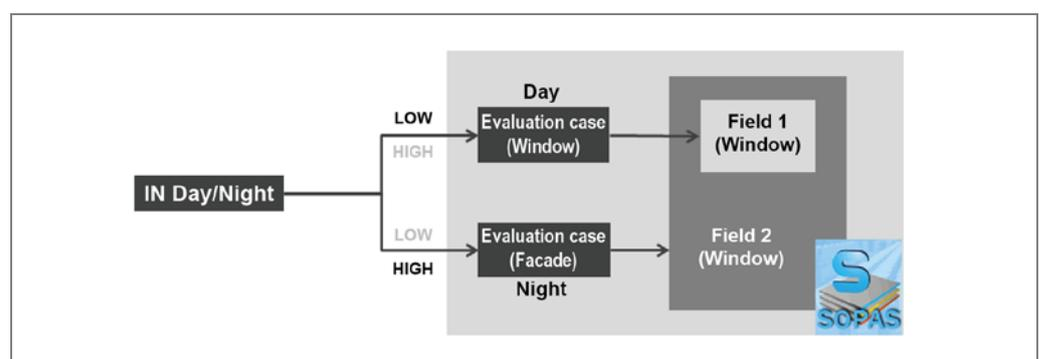
Fig. 58: Activating analysis cases (switching input Day/Night)
