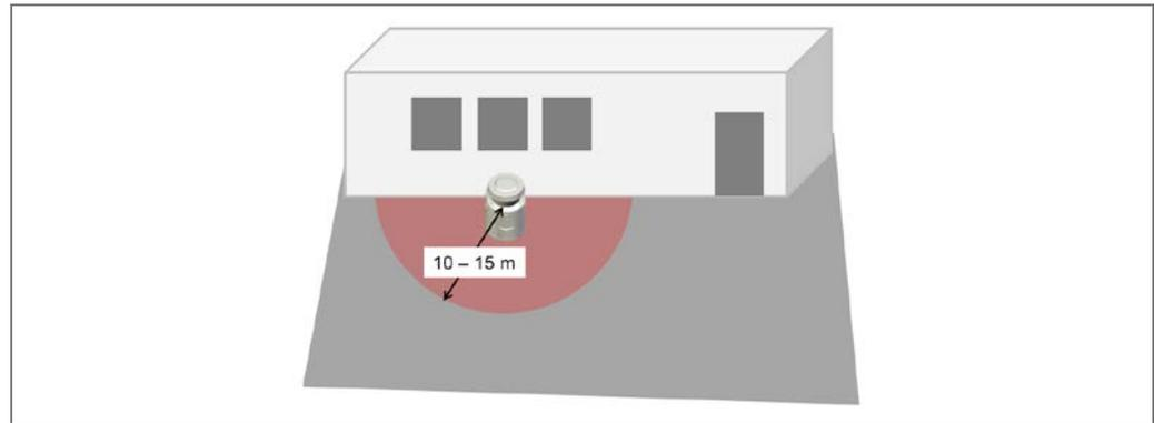
Fig. 92: LMS13x monitored area (open space protection)
