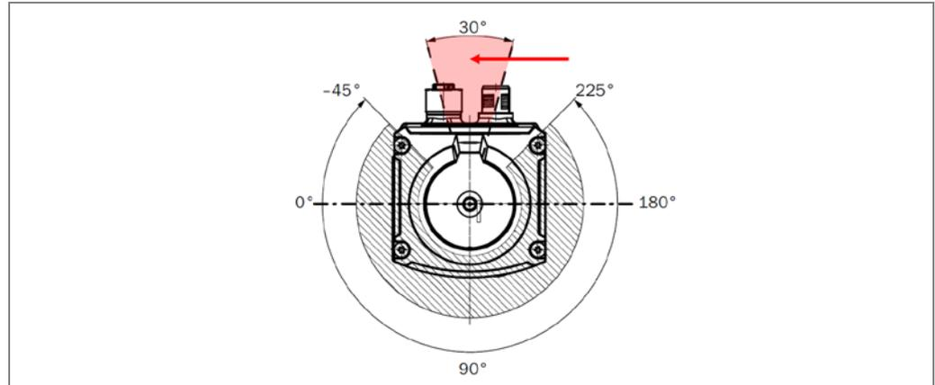
Fig. 23: Area behind the reference target in which no reflective surfaces are allowed
