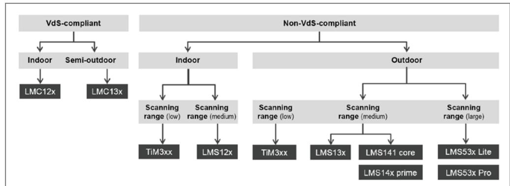
Fig. 20: Flowchart for device selection
