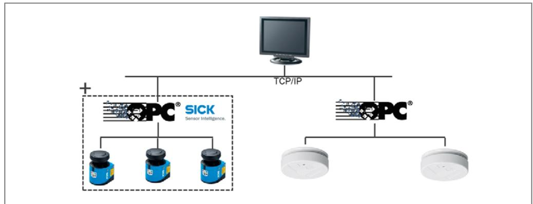
Fig. 79: Integration of laser scanners using SICK OPC server
