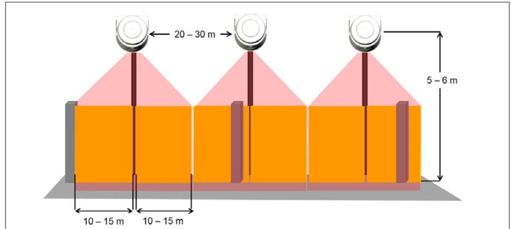
Fig. 83: LMS13x monitored area (fence protection)
