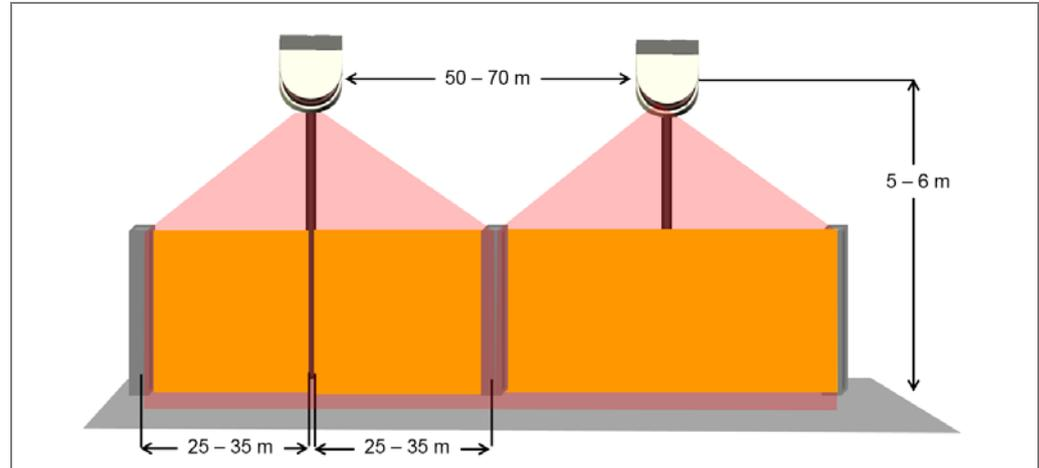
Fig. 81: LMS531 Lite/PRO monitored area (fence protection)
