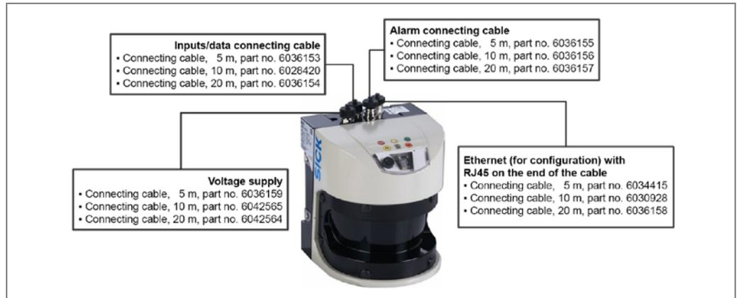
Fig. 75: LMS531 Lite connecting cables (with part number)
