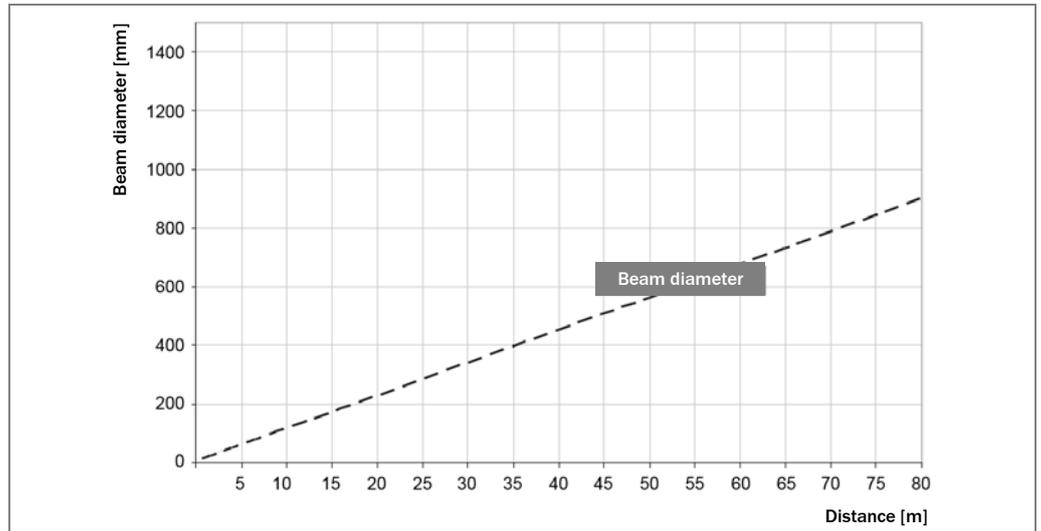
Fig. 11: LMS5xx beam diameter
