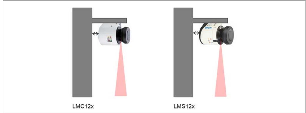
Fig. 95: LMC12x/LMS12x installation situation (painting protection)
