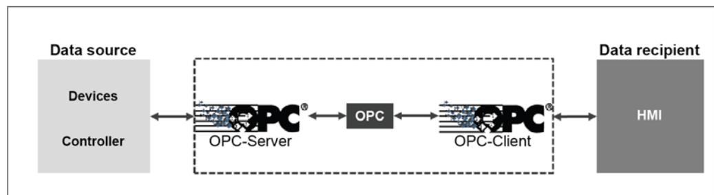
Fig. 78: OPC client/server architecture
