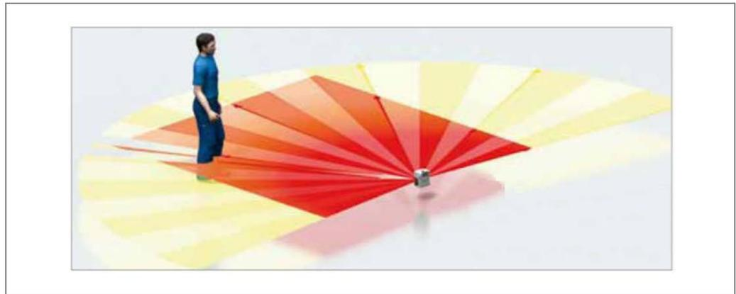
Fig. 1: 2D laser scanner principle of operation
