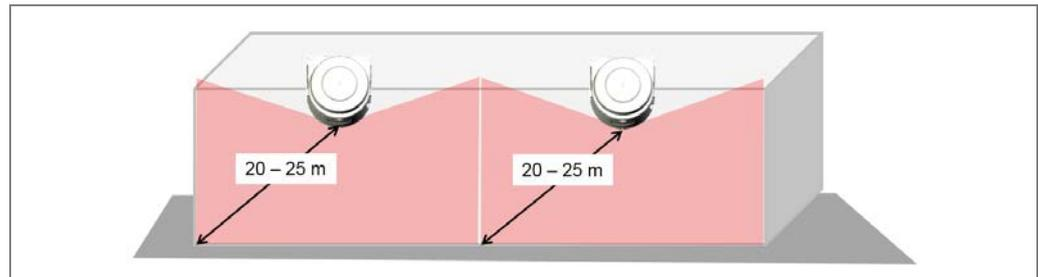
Fig. 86: LMS14x core/prime monitored area (facade protection)
