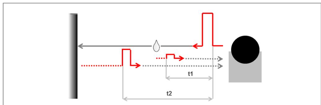
Fig. 34: Multi-echo analysis principle of operation
