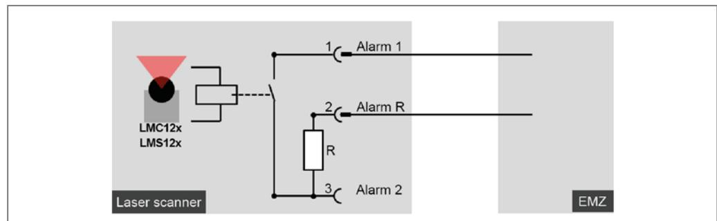
Fig. 63: Circuitry with resistance monitoring (LMC12x/LMS12x)
