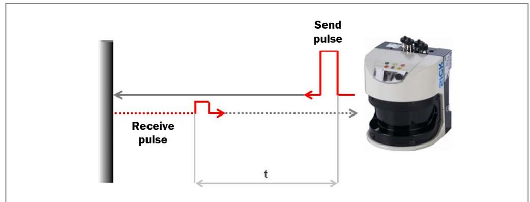
Fig. 2: Pulse time-of-flight measurement principle of operation
