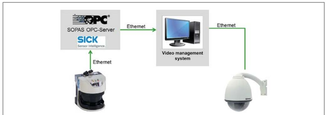
Fig. 70: Field-based camera control (via OPC)
