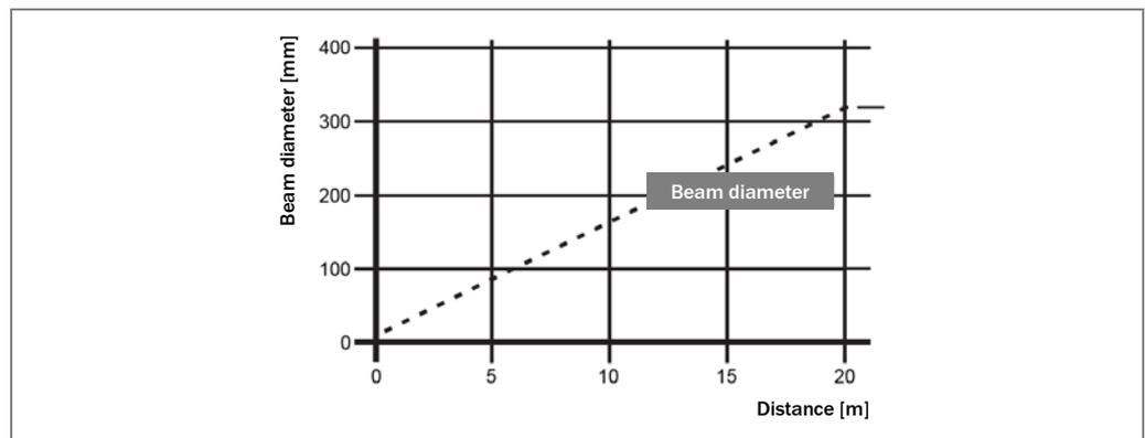
Fig. 9: LMS1xx beam diameter
