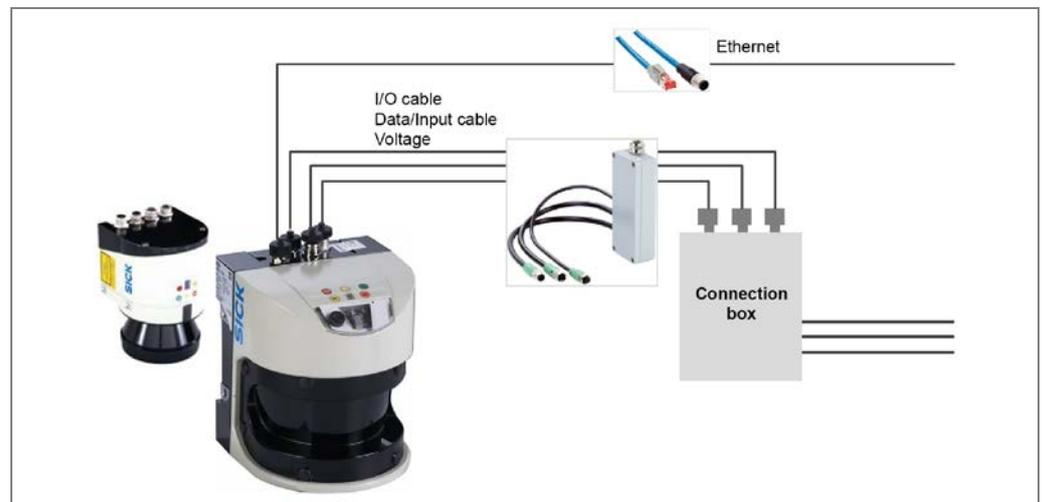
Fig. 31: Connection box for LMS13x/LMS141 core/LMS14x prime/LMS531 Lite
