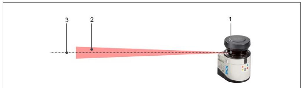
Fig. 8: LMS1xx beam expansion
