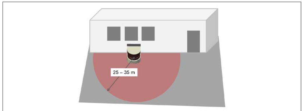
Fig. 90: LMS531 Lite/PRO monitored area (open space protection)
