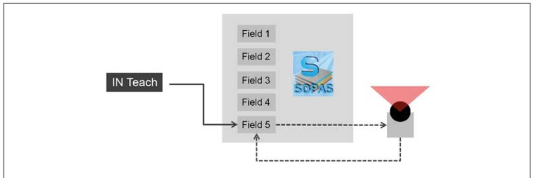
Fig. 52: Easy Teach PRO principle of operation
