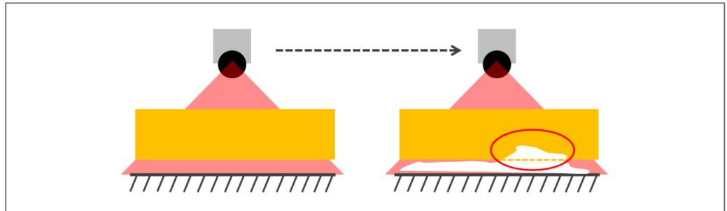
Fig. 46: Field breaches caused by changing ambient conditions
