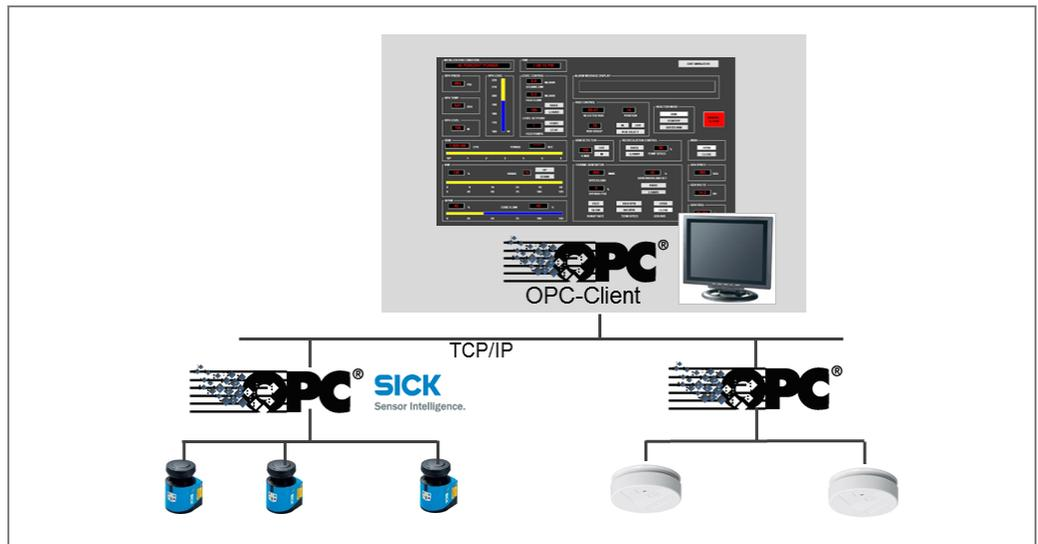
Fig. 80: Viewing information based on OPC
