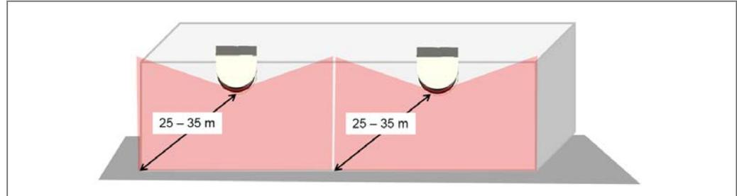
Fig. 85: LMS531 Lite/PRO monitored area (facade protection)
