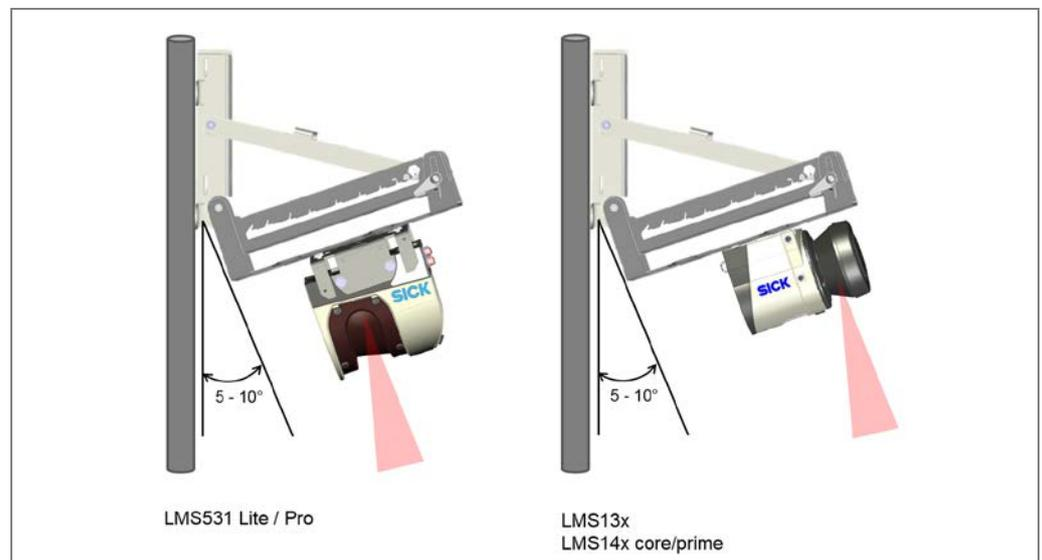
Fig. 84: Installation situation (fence protection)\*
