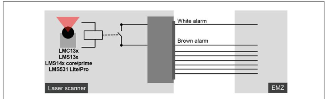
Fig. 62: Circuitry without resistance monitoring (LMC13x/LMS13x/LMS141 core/LMS14x prime/LMS531 Lite/LMS531 PRO)
