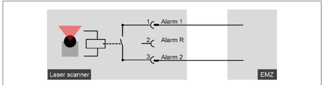
Fig. 61: Circuitry without resistance monitoring (LMC12x/LMS12x)
