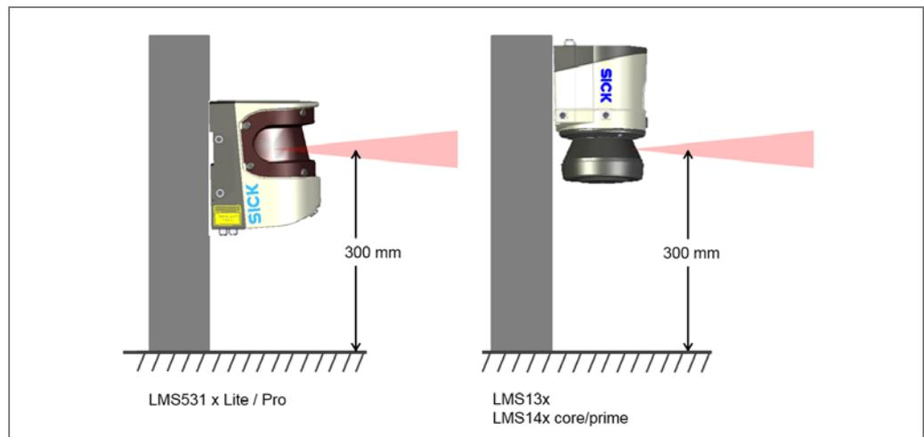
Fig. 93: Installation situation (open space protection)\*
