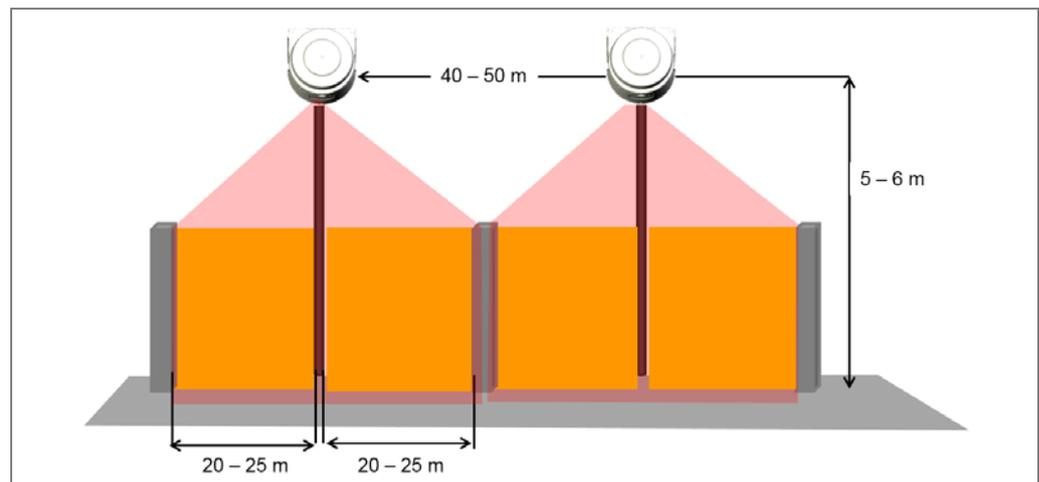
Fig. 82: LMS141 core/LMS14x prime monitored area (fence protection)
