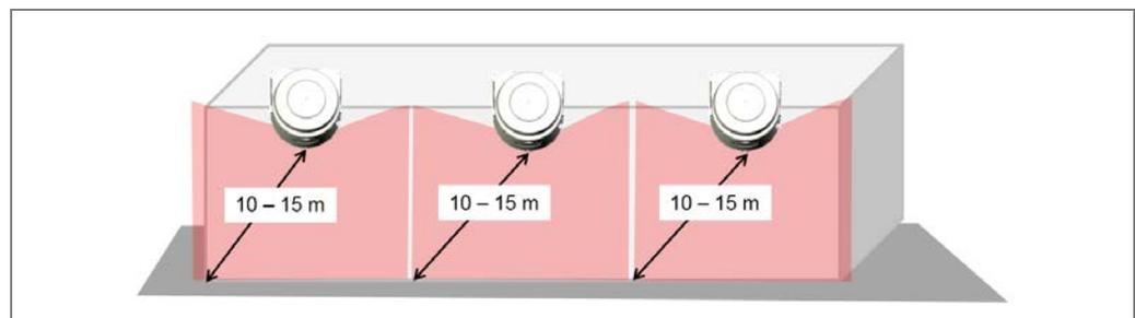
Fig. 87: LMS13x monitored area (facade protection)
