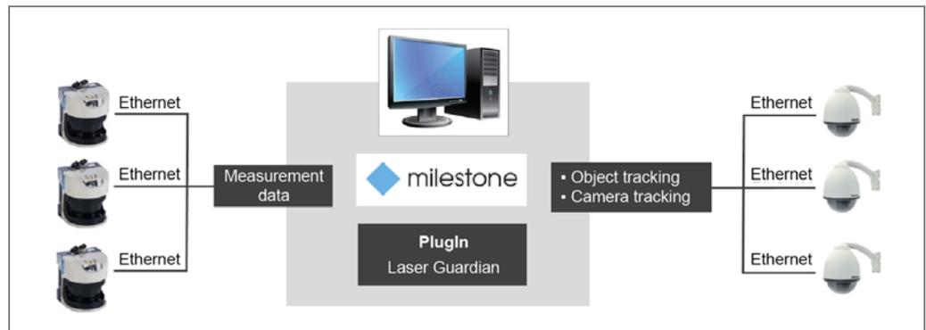
Fig. 71: How to integrate a laser scanner into Milestone XProtect
