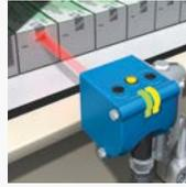
Countless manufacturers use self-adhesive seals (tamper evident labels) for cost-effective and easily-upgradeable tamper protection. Machines attach these seals over the insert flaps of folding boxes. The Glare sensor detects the presence of the labels. At the same time, it very reliably distinguishes between clear reflections from the plastic surface of the label and diffuse reflections from the surface of the packaging material.
