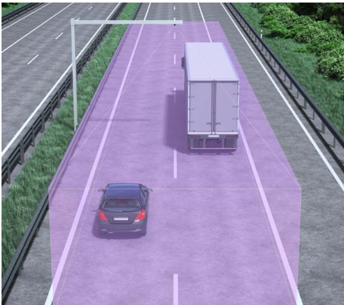
Profiling and tracking of vehicles across two lanes using a single sensor
