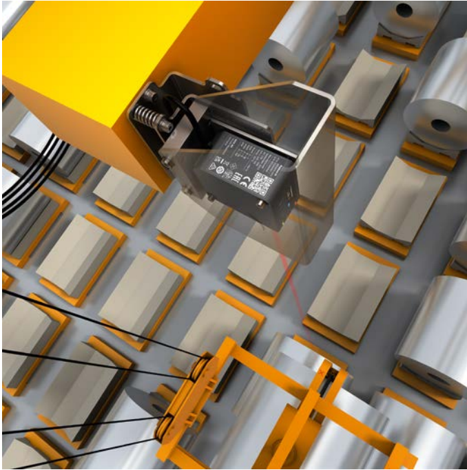
Positioning and collision avoidance of industrial cranes
