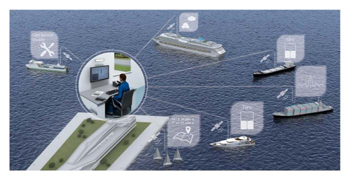
The TDC (Telematic Data Collector) gateway system is an open IIoT platform that links sensors and machines together for reliable network communication. As well as transmitting data to the target platform via a wired, mobile or wireless
