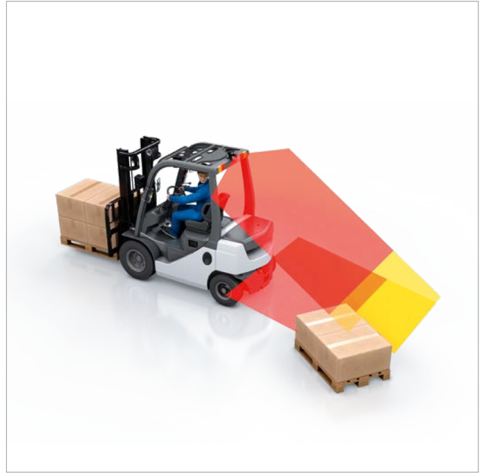
A system variant with two sensors is well suited for targeted coverage of blind spots.
