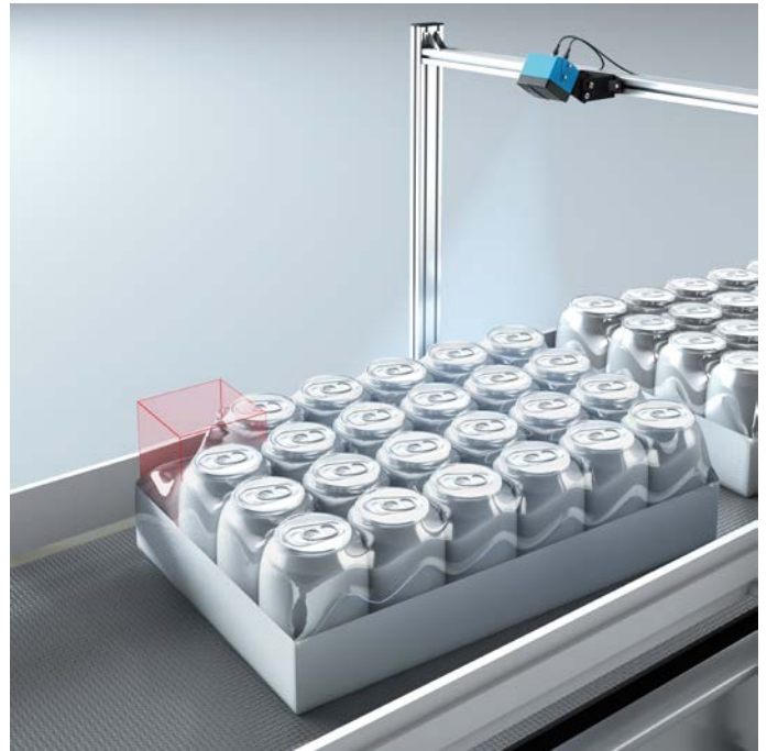
The Visionary-T Mini running SICK Nova Intelligent Inspection toolset ensure that objects in cartons, crates or pallets are positioned correctly, at right quantity and that unwanted objects are not present.
