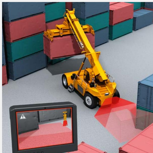
Figure 6: Visionary-B is also a valuable addition to agricultural and forestry machines. It can detect possible hazards and accidents in good time and send an active warning to the driver.
