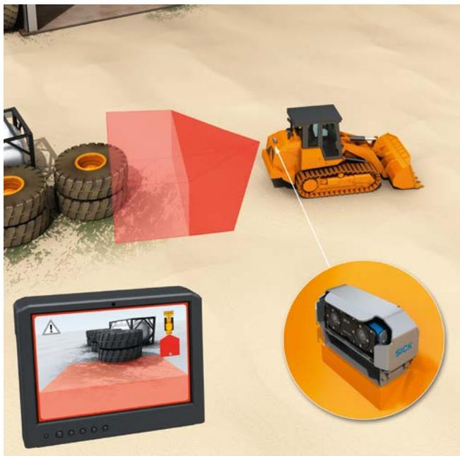
Figure 5: The Visionary-B 3D vision sensor reliably detects relevant objects in the driver's blind spot and issues a warning.
