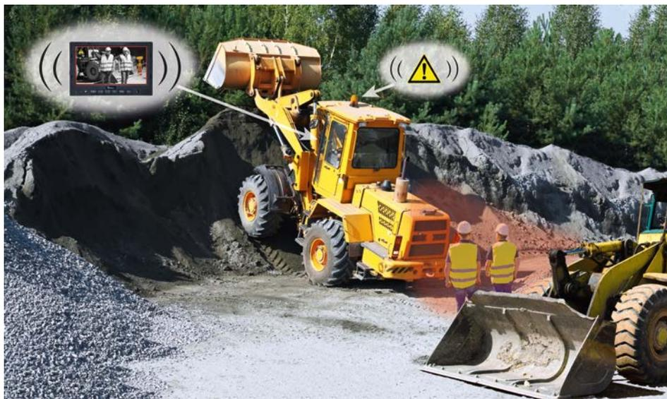
Figure 1: This system is a driver assistance system designed to enhance collision awareness, it should be used to support drivers. This product is not a safety component as defined in the Machinery Directive.
