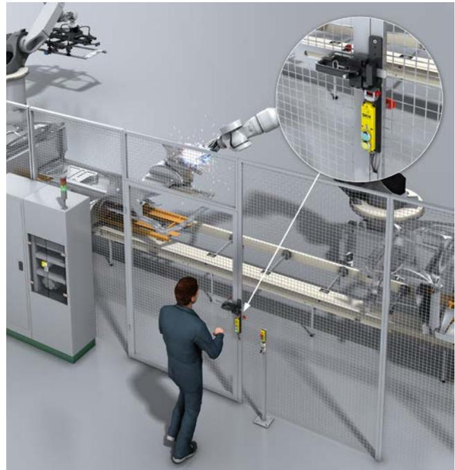
Protection of the access door for the welding robot
