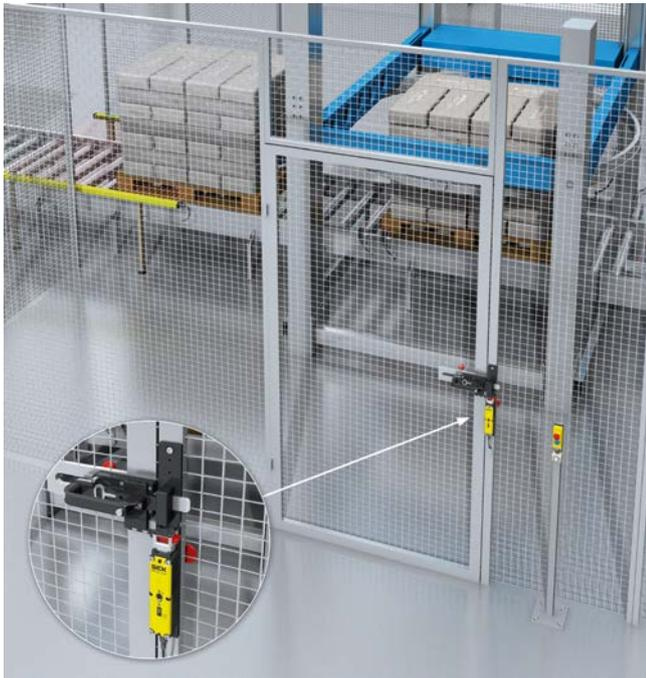
Protection of the access door for the stretch film wrapper
