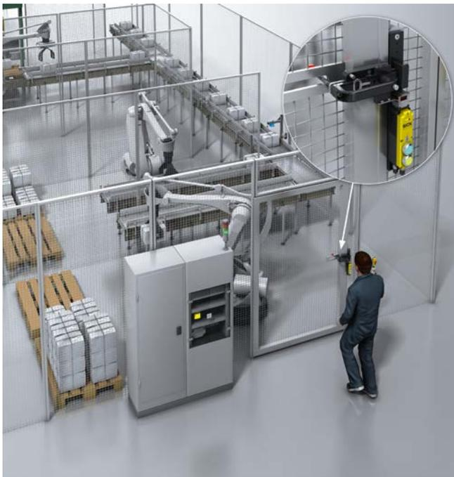
Protection of the access door for the stacker robot
