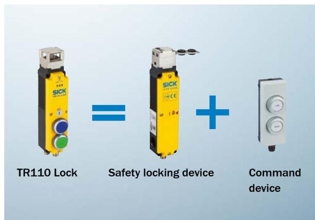
A further variant of the TR110 Lock is characterized by its integrated display and control elements. Illuminable pushbuttons or indicator lights in the switch cover make it possible to trigger control signals such as door requests or acknowledgments, directly on the safety switch. There is no need for an additional command device.
