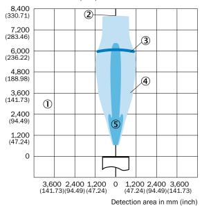
$\ensuremath{ \textcircled{1}}$  Detection range dependent on reflection properties, size, and alignment of the object
