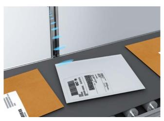
Detecting very flat objects which are difficult to detect optically using edge detection maximizes productivity
