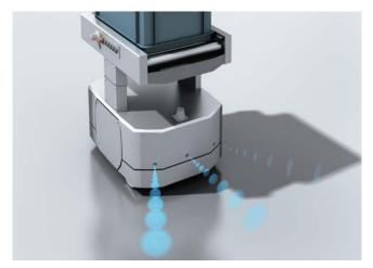
Detecting obstructions over a large area in order to control and brake automated guided vehicle enables a high level of automation
