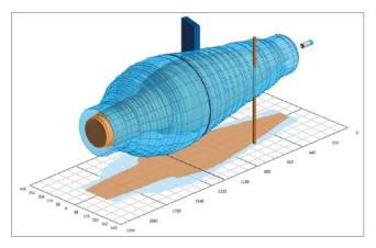
Sound cone adjustment with live measurement value visualization in SOPAS ET - 3D
