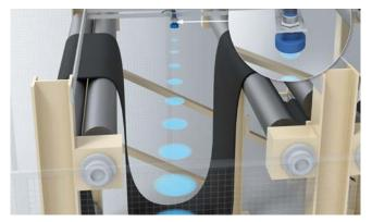
Adjusting the material feed according to the slack depth improves the process quality
