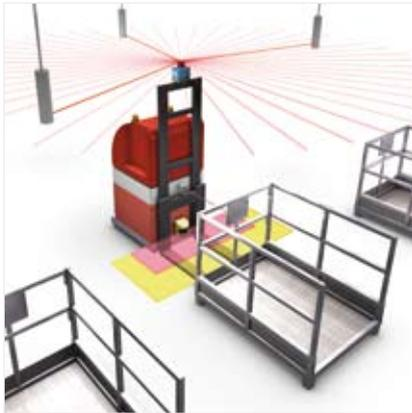
◀ The DT50 distance sensor continuously measures the distance between the AGV and the load to be picked up (grid box) in order to adapt the vehicle's speed. It supplies the signal for lifting when the load has been correctly positioned on the hoisting fork.
