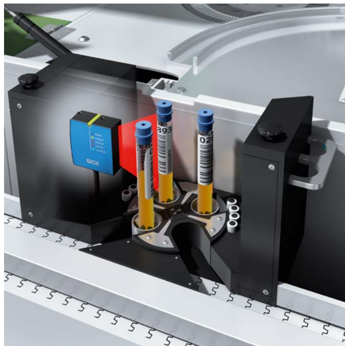
Sample identification in laboratory Automation
