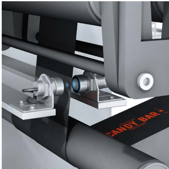
Accurate double layer detection when splicing film
