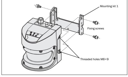
Fig. 28: Mounting with mounting kit 1 (part no. 2015623)
