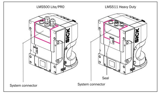
Fig. 63: Disassemble the system connector
