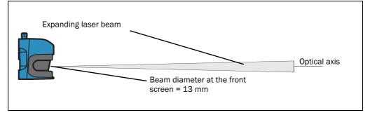
Fig. 13: Beam expansion
