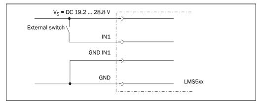
Fig. 54: Connecting digital inputs as non-floating
