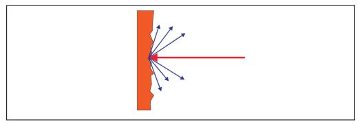
Fig. 7: Reflection of the laser beam at the surface of an object
