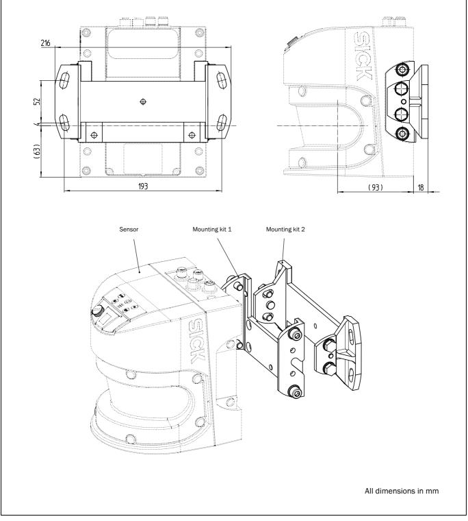
Fig. 69: Dimensional drawing, mounting kit 2
