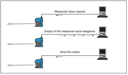
Fig. 18: Continuous measured value output
