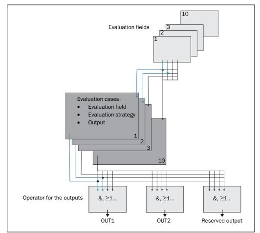
Fig. 22: Principle of the field application
