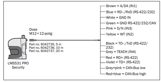
Fig. 52: LMS531 PRO Security: "Inputs" connection
