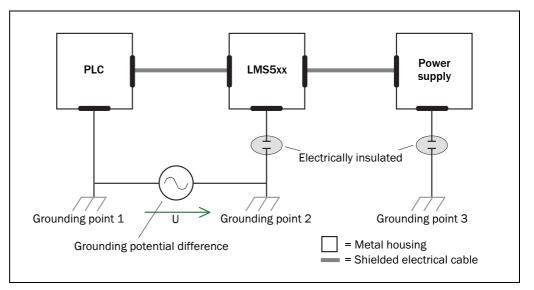
Fig. 42: Insulated assembly of the LMS5xx and the peripheral devices (sample)
