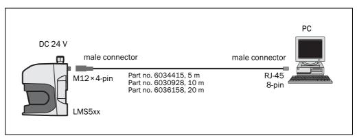
Fig. 44: LMS5xx: Ethernet connection using the Ethernet cable
