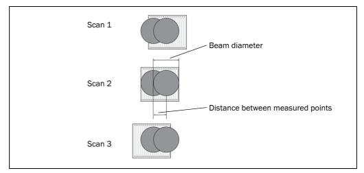
Fig. 16: Minimum object size for detection
