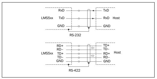
Fig. 61: Wiring of the RS-232 or RS-422 interface
