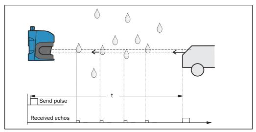
Fig. 19: Principle of operation of the measurement of the fifth received echo (LMS5xx PRO/Heavy Duty)
