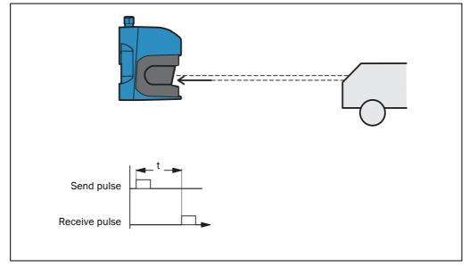
Fig. 6: Principle of operation for time of flight measurement
