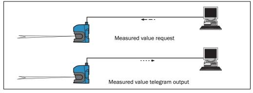
Fig. 17: Measured value telegram request
