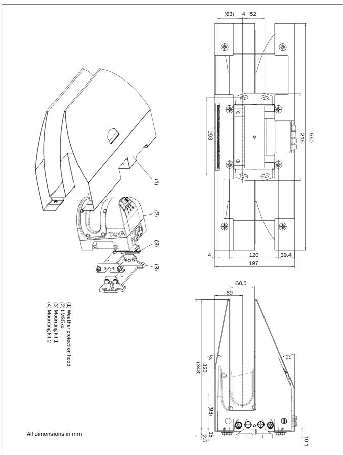
Fig. 72: Dimensional drawing weather protection hood
