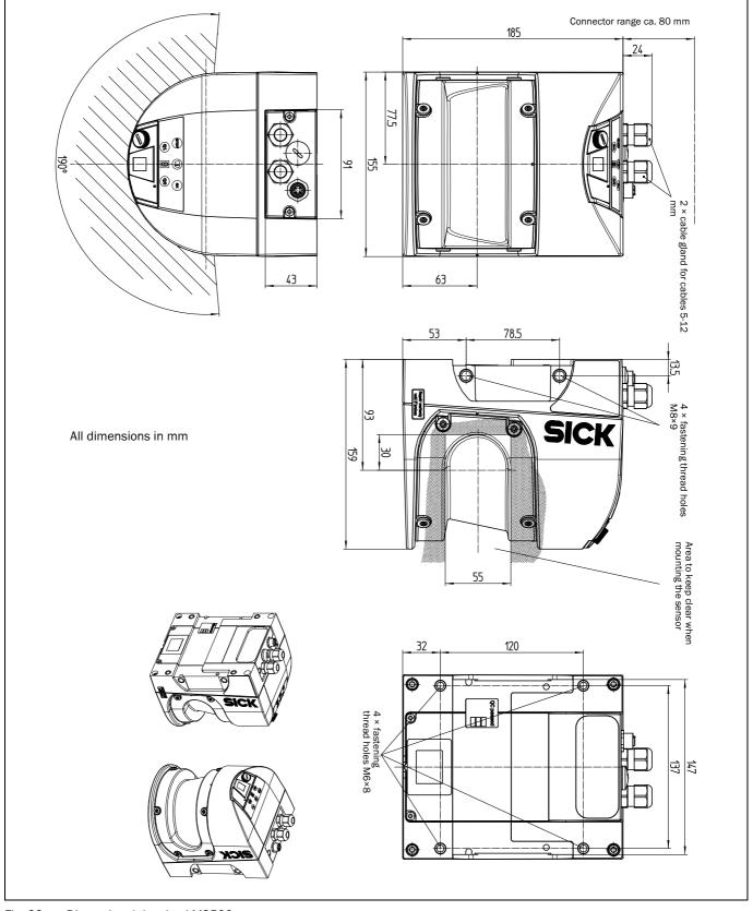
Fig. 66:Dimensional drawing LMS500
