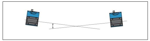
Fig. 35: Crosswise placement of two LMS5xx
