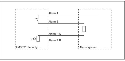
Fig. 60: Resistance-monitored connection of the outputs of the LMS531 Security to an alarm system
