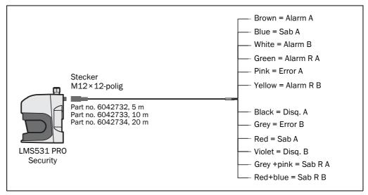
Fig. 53: LMS531 PRO Security: "Alarm" connection"
