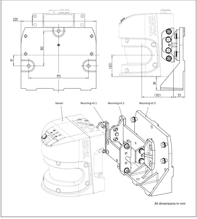
Fig. 70: Dimensional drawing, mounting kit 3 (mm)
