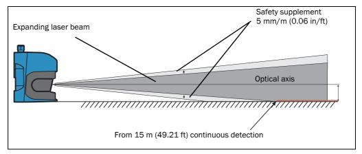
Fig. 26: Increase in the size of the beam and safety supplement
