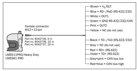
Fig. 48: LMS511 PRO/LMS581 PRO Security/LMS511 Heavy Duty: "Data" connection
