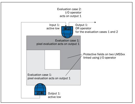
Fig. 25: Logical operators for inputs and outputs
