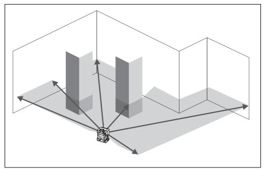
Fig. 5: Measuring principle of the LMS5xx
