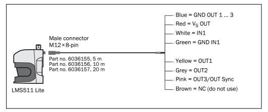
Fig. 47: LMS511 Lite: "I/O" connection
