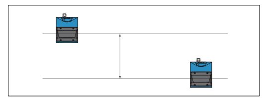
Fig. 36: Placement of two LMS5xx with parallel offset
