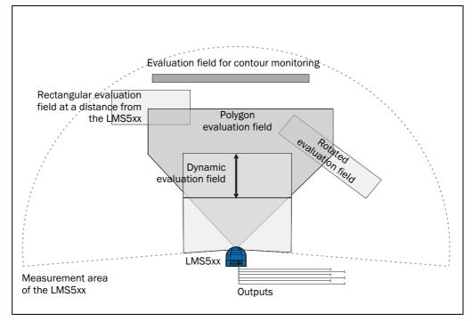
Fig. 24: Examples of 4 different evaluation field shapes
