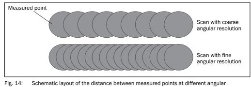
Fig. 14: Schematic layout of the distance between measured points at different angular resolutions
