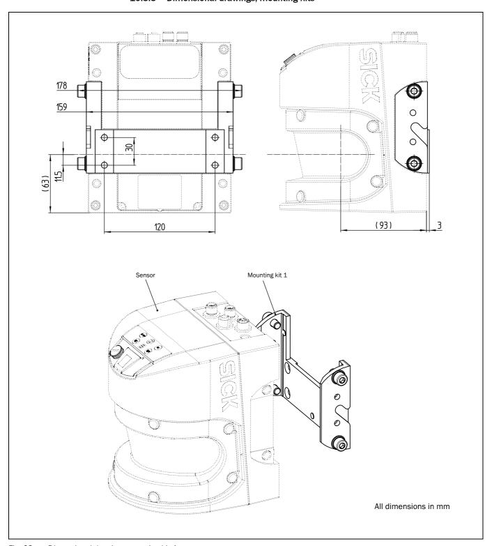
Fig. 68: Dimensional drawing, mounting kit 1
