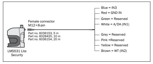
Fig. 50: LMS531 Lite Security: "Inputs" connection
