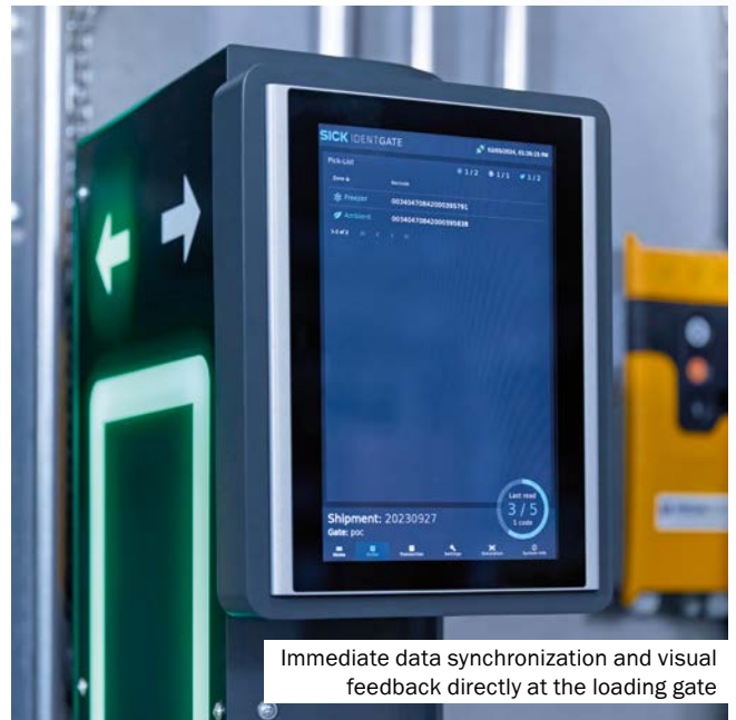
Automatic and technology-independent capture of the transport label
