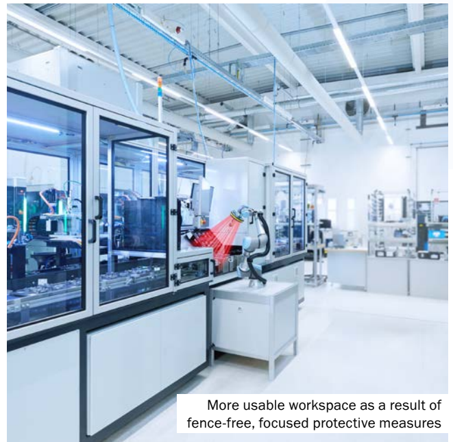
Faster cobots thanks to protection of the tool and workpiece area
