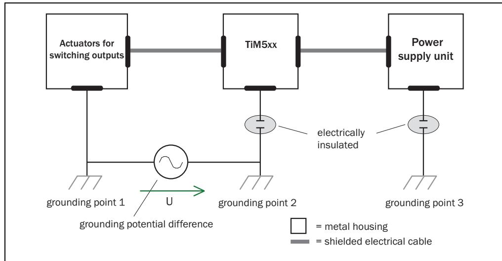
There is effective suppression of ground loops even at ground potential differentials of up to 60 V RMS / 80 V DC maximum. As result, equalizing currents can no longer flow via the cable shields and metal housing.
