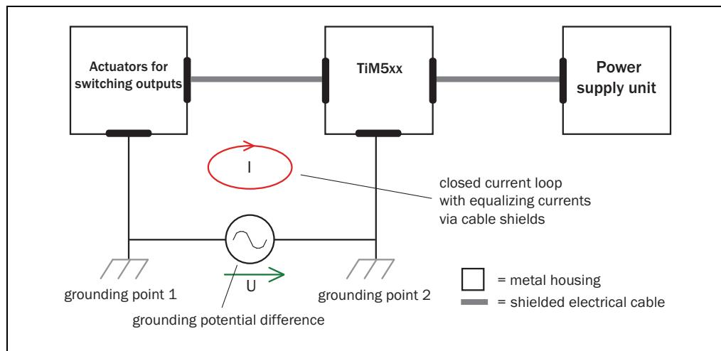
Insufficient ground potential equalization leads to voltage differences arising between grounding points 1 and 2. The current loop closes via the shielded cables/metal housing.
