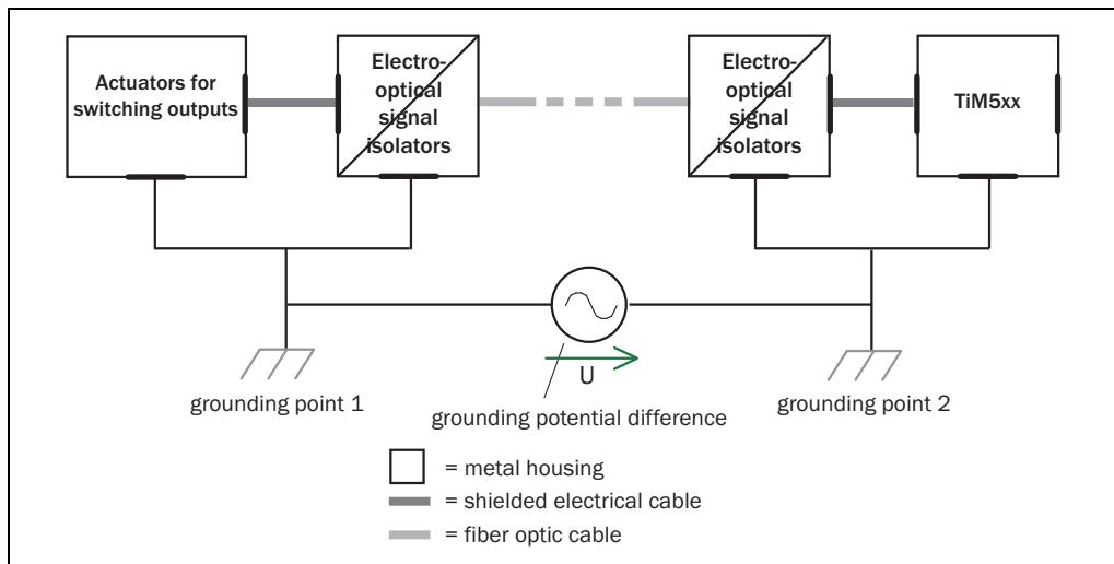
The ground loop is isolated by using the electro-optical signal isolator between the islands. Equalization currents are prevented on the cable shields within the islands by conductible equipotential bonding.
