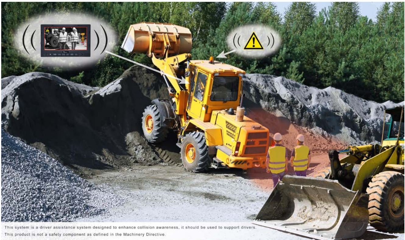
Figure 10: Typical environment in construction site. The 3D snapshot sensor from SICK helps the operator to focus on his main tasks. The sensor actively warns the operator in critical situations with an acoustic and visual alarm.
