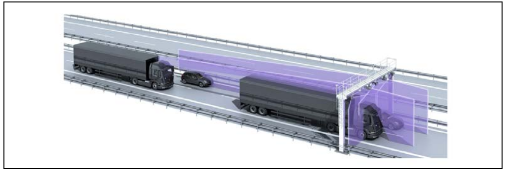
Fig. 11: Operating principle of vehicle detection
