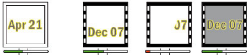
Figure – The Edge pixel counter counts pixels that are edges and compares this number with the No. of edge pixels settings. Where the pixels are located does not matter.
