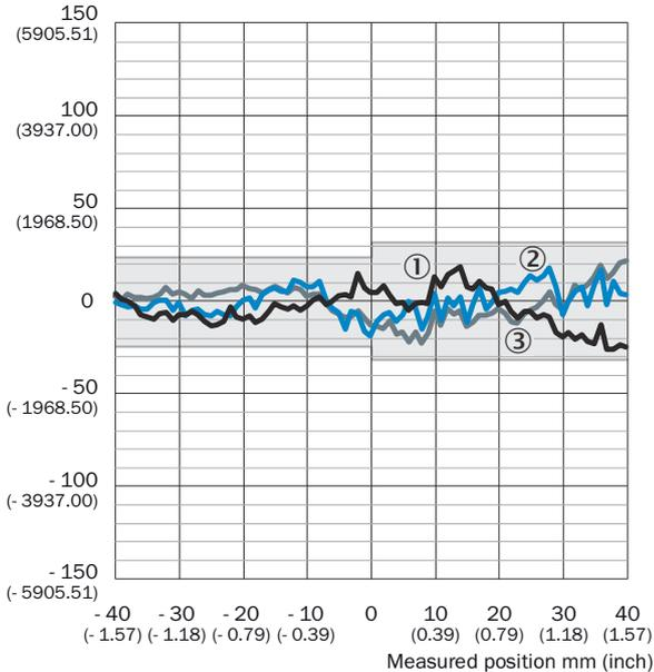
Figure 72: Linearity OD5000-C150Txx (diffuse reflection)
