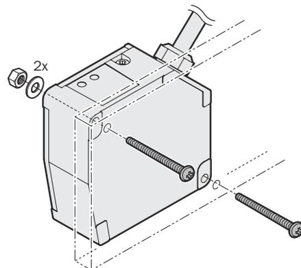
Figure 18: Mounting on the wall
