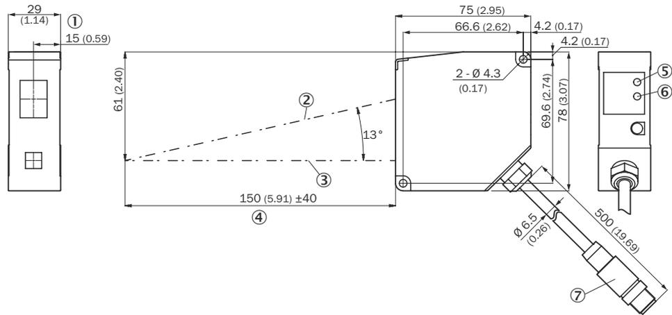
Figure 7: OD5000-C150xxx: Structure and dimensions, unit: mm (inch), decimal separator: period
