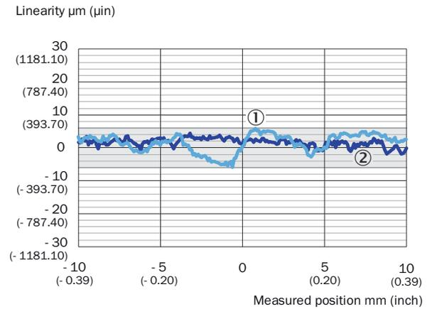
Figure 69: Linearity OD5000-C85Txx (specular reflection)
