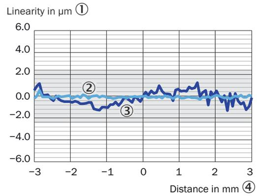
Figure 67: Linearity OD5000-30Wxx (specular reflection)
