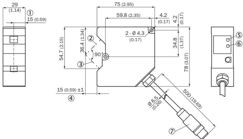
Figure 4: OD5000-C15xxx: Structure and dimensions, unit: mm (inch), decimal separator: period
