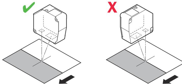
Figure 22: Mounting with different material or colors
