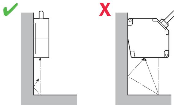
Figure 25: Mounting on the wall
