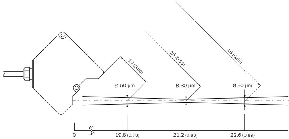
Figure 9: Typical light spot size of the OD5000-C15T01, unit for distance values: mm (inch), decimal separator: period
