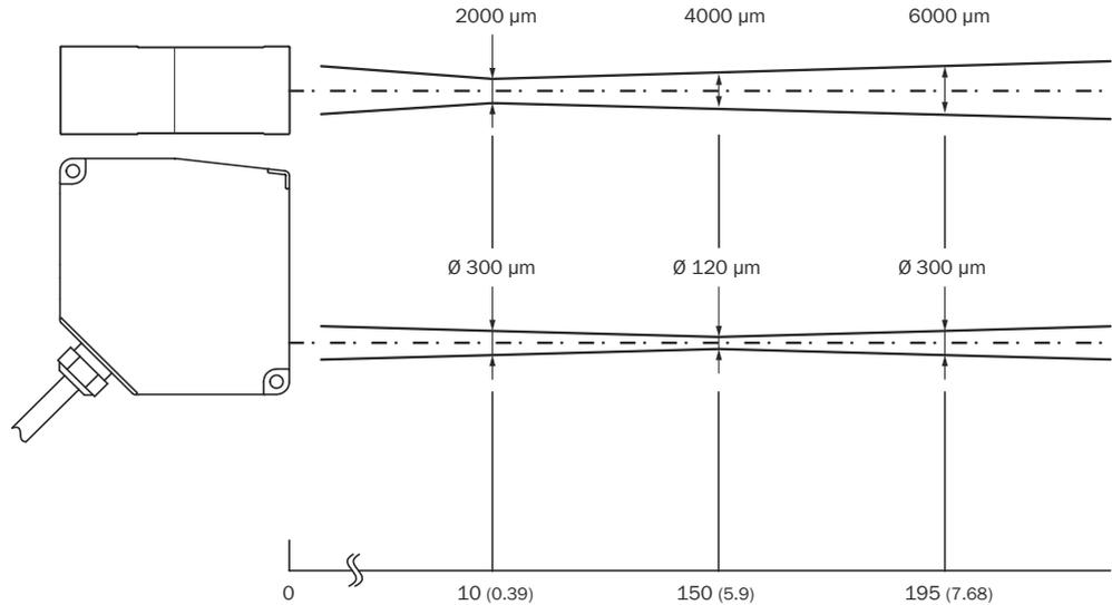
Figure 16: Typical light spot size of the OD5000-C150W40, unit for distance values: mm (inch), decimal separator: period
