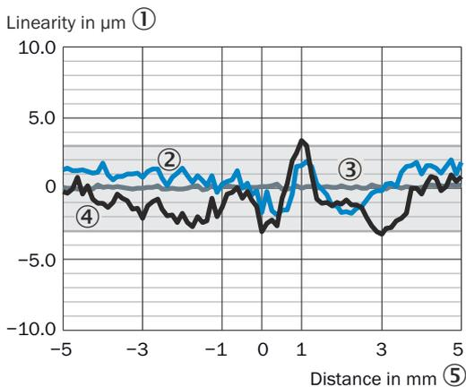
Figure 64: Linearity OD5000-C30Txx (diffuse reflection)
