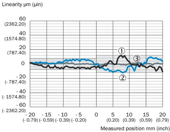
Figure 68: Linearity OD5000-C85Txx (diffuse reflection)
