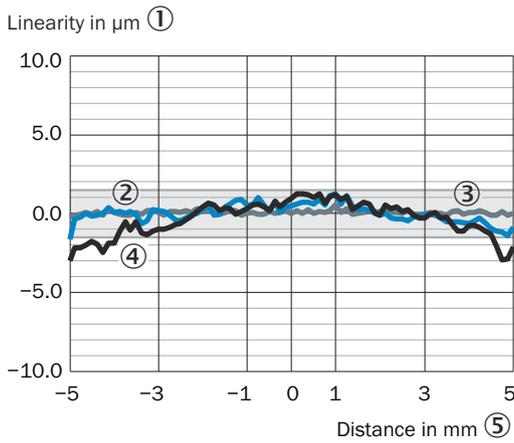
Figure 66: Linearity OD5000-30Wxx (diffuse reflection)
