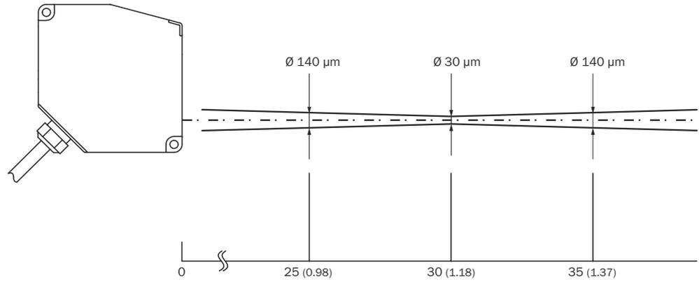
Figure 11: Typical light spot size of the OD5000-C30T05, unit for distance values: mm (inch), decimal separator: period
