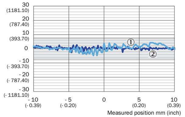
Figure 71: Linearity OD5000-C85Wxx (specular reflection)
