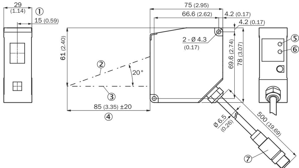
Figure 6: OD5000-C85xxx: Structure and dimensions, unit: mm (inch), decimal separator: period
