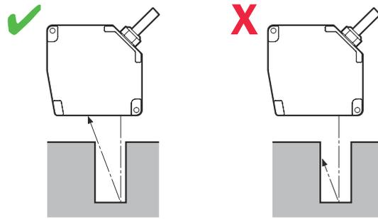
Figure 24: Mounting with holes or recesses
