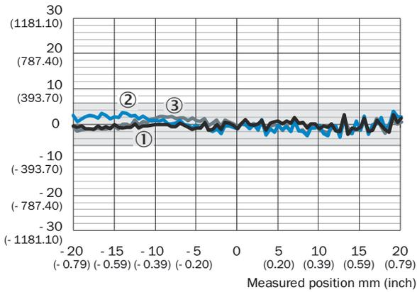
Figure 70: Linearity OD5000-C85Wxx (diffuse reflection)
