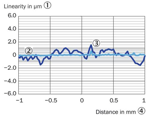
Figure 63: Linearity OD5000-C15Wxx (specular reflection)
