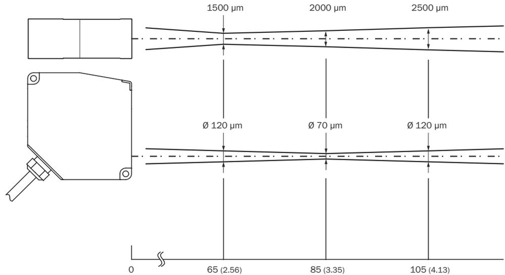
Figure 14: Typical light spot size of the OD5000-C85W20, unit for distance values: mm (inch), decimal separator: period
