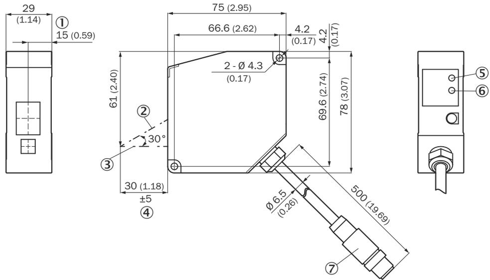
Figure 5: OD5000-C30xxx: Structure and dimensions, unit: mm (inch), decimal separator: period
