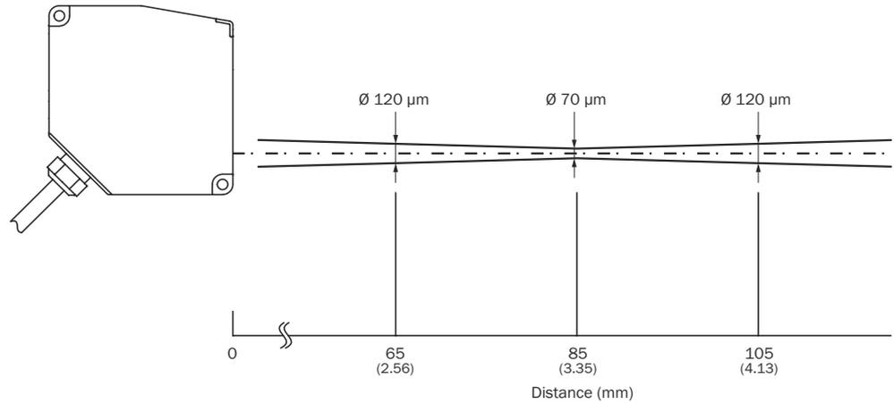
Figure 13: Typical light spot size of the OD5000-C85T20, unit for distance values: mm (inch), decimal separator: period
