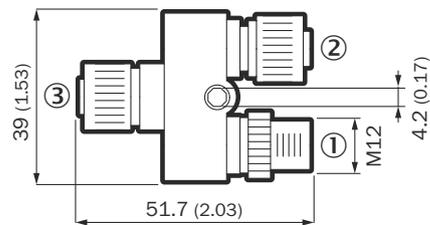
Figure 8: Y adapter: Structure and dimensions, unit: mm (inch), decimal separator: period
