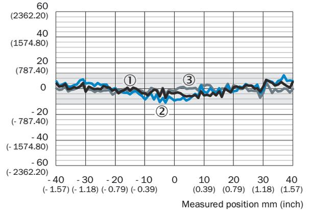
Figure 73: Linearity OD5000-C150Wxx (diffuse reflection)
