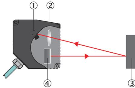
Figure 3: Triangulation principle
