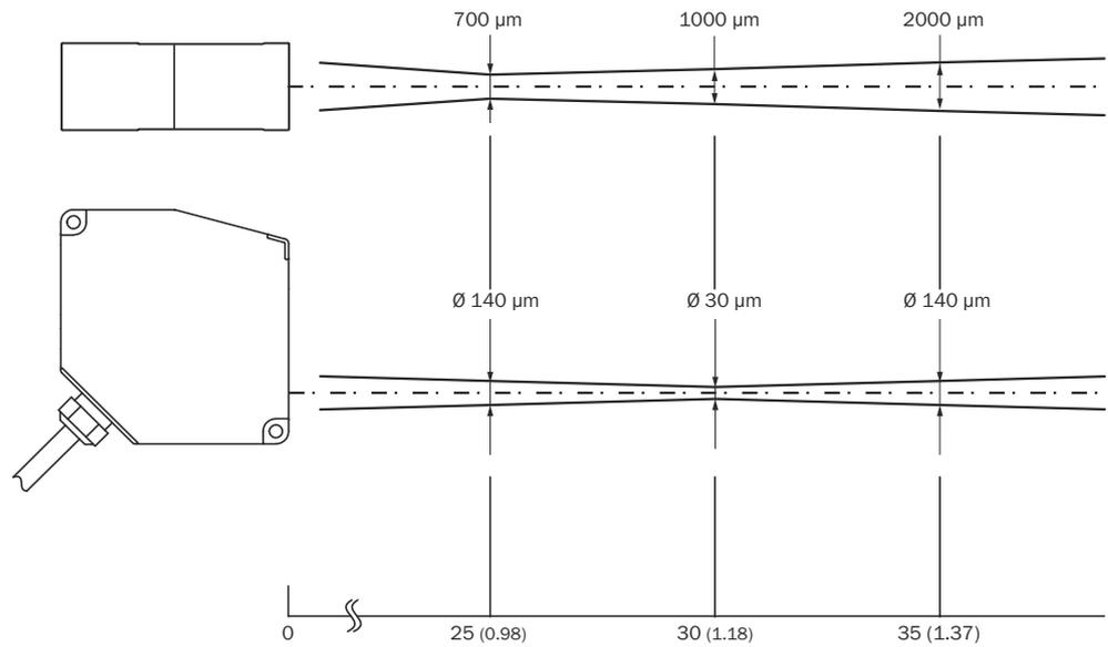
Figure 12: Typical light spot size of the OD5000-C30W05, unit for distance values: mm (inch), decimal separator: period
