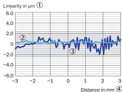
Figure 65: Linearity OD5000-C30Txx (specular reflection)
