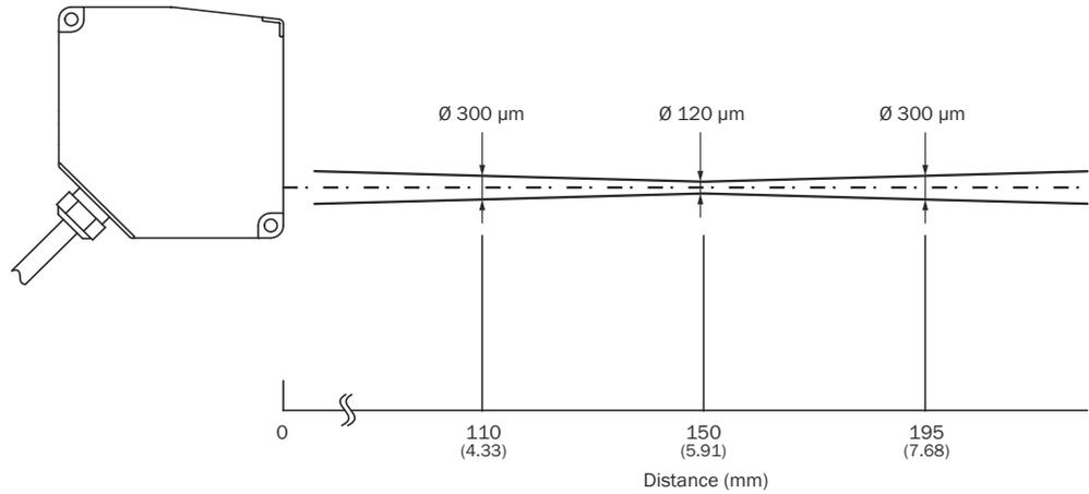
Figure 15: Typical light spot size of the OD5000-C150T40, unit for distance values: mm (inch), decimal separator: period
