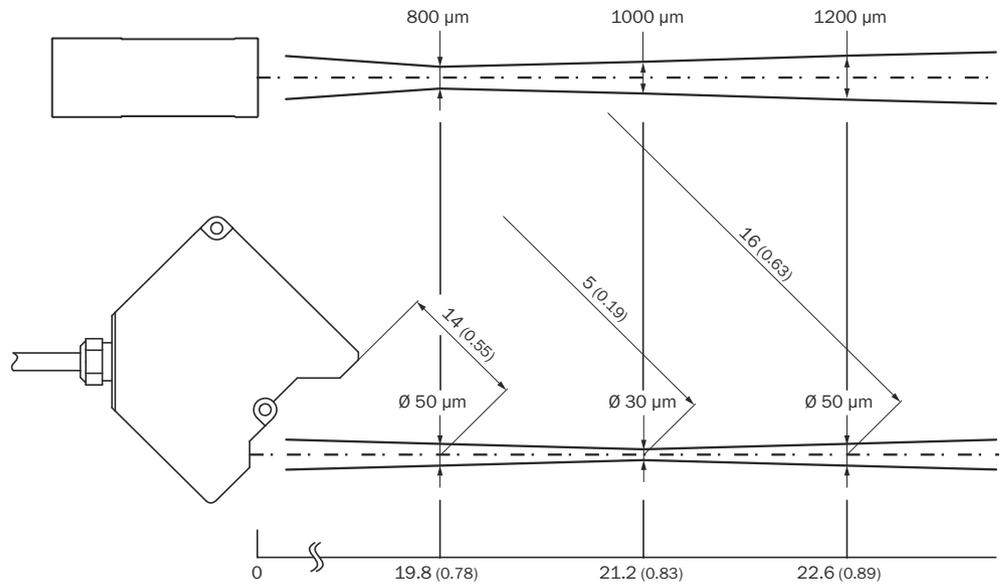
Figure 10: Typical light spot size of the OD5000-C15W01, unit for distance values: mm (inch), decimal separator: period
