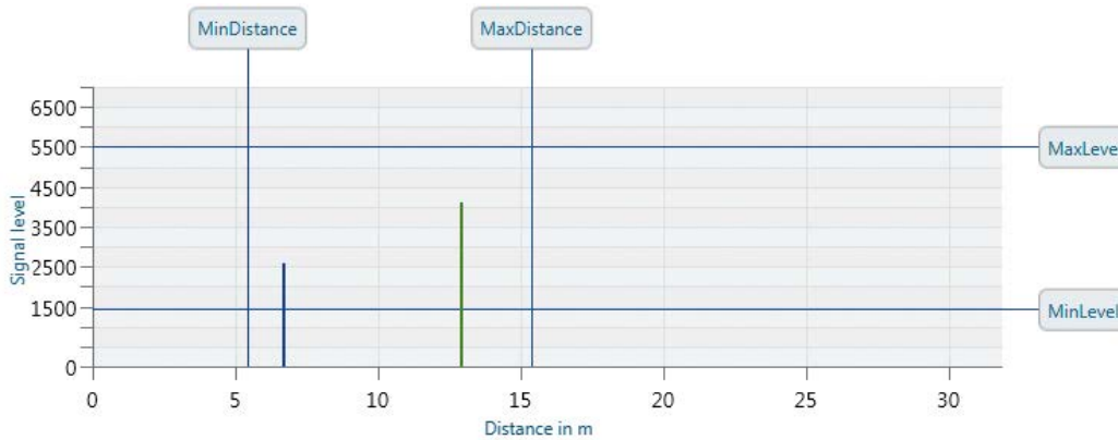
Fig. 4: Diagram defining the region of interest of the Dx1000 distance sensor from SICK.
