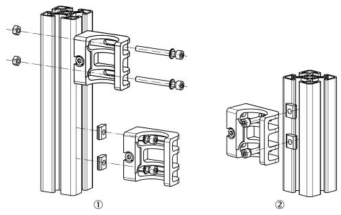
Figure 21: Mount FlexFix brackets to a profile frame
