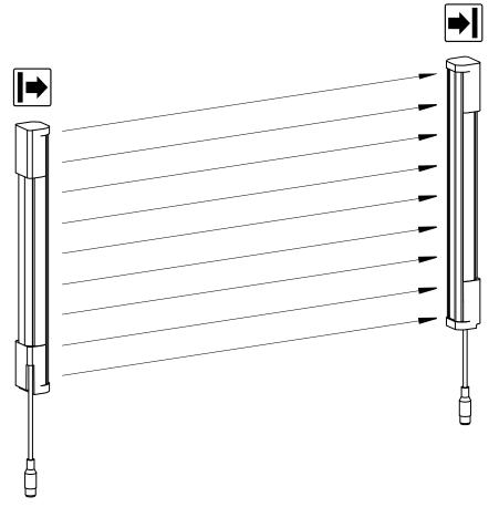
Figure 1: Sender and receiver
