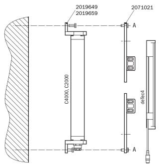
Figure 24: Upgrade bracket, installation version A
