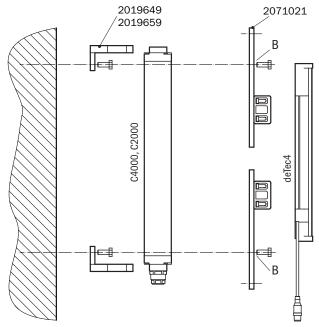
Figure 25: Upgrade bracket, installation version B
