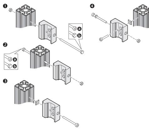
Figure 20: Mounting the QuickFix bracket to a profile
