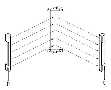
Figure 37: Example of use of deflector mirrors
