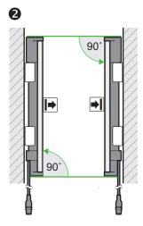
Position the brackets near the ends of the housing. For devices with a protective  $\blacktriangleright$ field height > 300 mm, the distance between the bracket and the end of the housing must not exceed 1/4 of the length of the housing. If the device is exposed to strong vibrations during operation, mount the top bracket at a height where the offset in the safety light curtain housing rests on the bracket (3).
