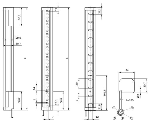
Figure 32: Dimensional drawing, sender and receiver
