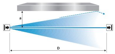
Figure 9: Minimum distance from reflective surfaces
