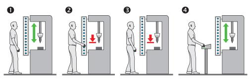
Figure 15: Schematic representation of operation with restart interlock
