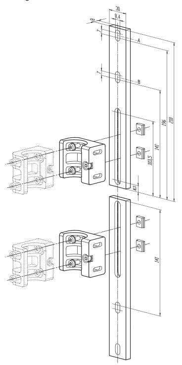
Figure 35: Dimensional drawing of the upgrade bracket (2071021)
