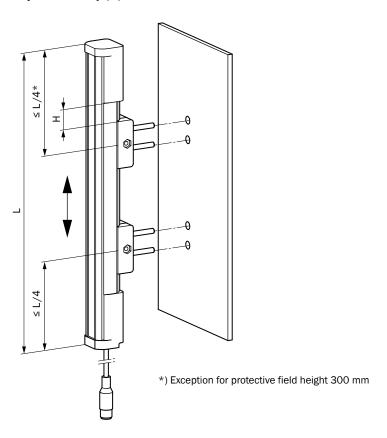
Figure 30: QuickFix bracket: adjust vertically
