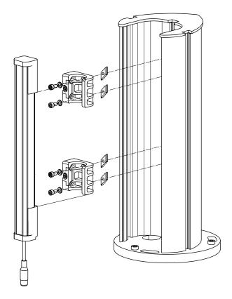
Figure 23: Mounting the FlexFix bracket on a device column (accessory)
