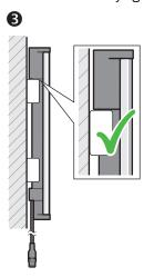
Tightening torque for the screws used to mount the bracket: 5 Nm ... 6 Nm. Tightening torque for the screws used to secure the safety light curtain in the bracket: 2.5 Nm ... 3 Nm (4). Higher torques can damage the bracket, while lower torques are not secure enough to prevent the safety light curtain from moving.
