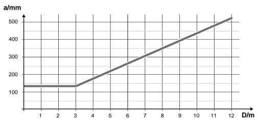
Figure 10: Graph of minimum distance from reflective surfaces
