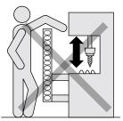
Figure 8: Representation of the accessibility of electro-sensitive protective device by reaching over. Left: Protective field that cannot be reached over. Right: Protective field that can be reached over.
