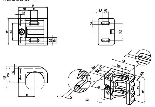
Figure 34: Dimensional drawing of the FlexFix bracket (2066614)
