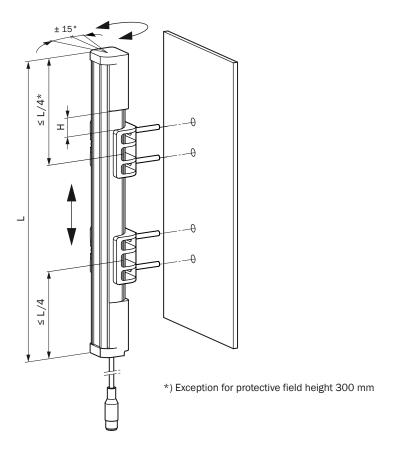
Figure 31: FlexFix bracket: adjust vertically/rotate
