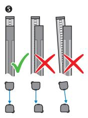
If necessary, use a spirit level to check that the components are parallel (6).
