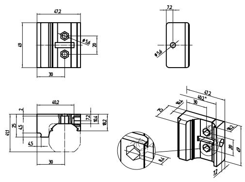
Figure 33: Dimensional drawing of the QuickFix bracket (2066048)
