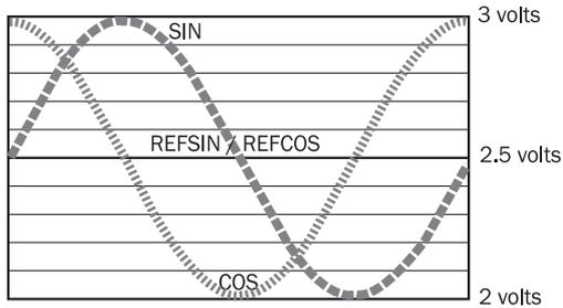
Diagrams Signal specification of the process channel
