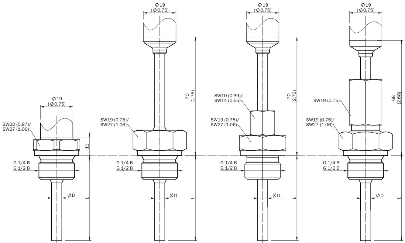
Process connections, cylindrical thread
