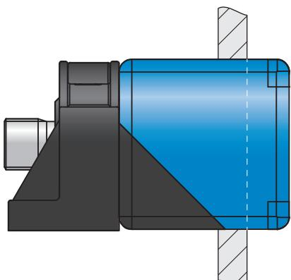
Recommended overrun of the active head when mounting the device in metal: about 10 mm (non-flush installation)
