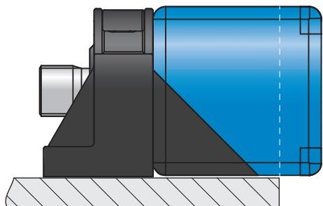
Recommended overrun of the active head when mounting the device on metal: about 10 mm
