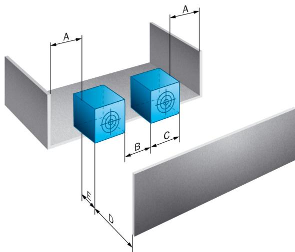
Distances required to prevent mutual interference with parallel mounting of several devices as well as from the environment.
