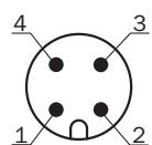
IO-Link connection (male connector, M12, 4-pin, A-coded)
