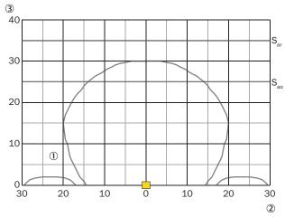
If the actuator moves laterally in relation to the surface of the sensor, a minimum distance of 3 mm must be maintained. This distance will prevent premature triggering due to the side approach areas.
