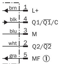
① multifunctional input/synchronization and multiplex operation/communication Connect+
