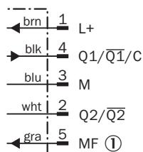
① multifunctional input/synchronization and multiplex operation/communication Connect+
