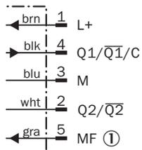
① multifunctional input/synchronization and multiplex operation/communication Connect+
