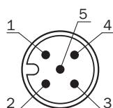
Connection diagram UM18-21xxxCxxx\_Dxxx, male connector M12, 5-pin
