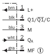
① multifunctional input/synchronization and multiplex operation/communication Connect+
