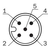
Connection diagram UM18-21xxxCxxx\_Dxxx, male connector M12, 5-pin
