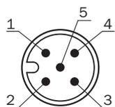
Connection diagram UM18-21xxxAxxx\_Bxxx, male connector M12, 5-pin
