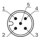
Connection diagram UM18-21xxxAxxx\_Bxxx, male connector M12, 5-pin
