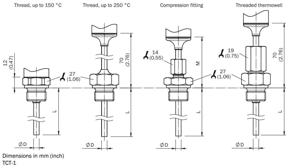
Connection type Round connector M12 x 1, output signal Pt100
