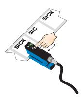
Press the teach-in button for 3 - 20 s. With the pushbutton pressed down, move several label with carrier material (label) through the sensor. The yellow LED flashes at 3 Hz during the teach-in procedure. Recommendation: Move at least 3 label + carrier through the sensor.
