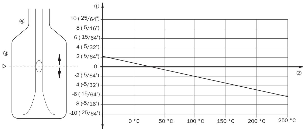
① Shifting of the switching point in mm (in)
