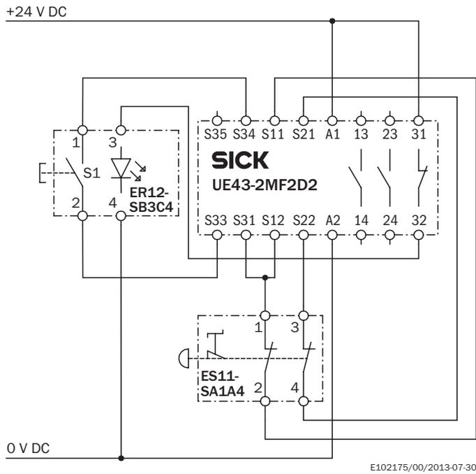
Connection diagram ER12 reset pushbutton and series connection of three ES11 emergency stop pushbutton to a Flexi Soft safety controller
