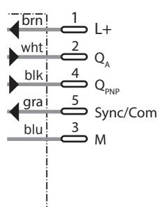
Connection type Plug, M12, 5-pin
