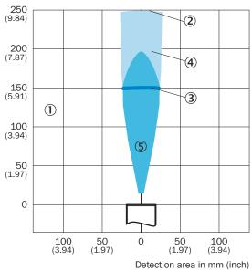
① Detection range dependent on reflection properties, size, and alignment of the object
