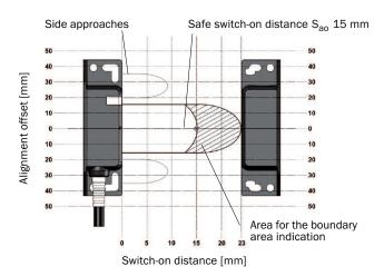
If the actuator moves laterally in relation to the surface of the sensor, a minimum distance of 9 mm must be maintained. This distance will prevent premature triggering due to the side approach areas. Pin assignment
