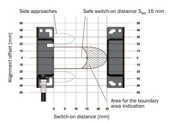
If the actuator moves laterally in relation to the surface of the sensor, a minimum distance of 9 mm must be maintained. This distance will prevent premature triggering due to the side approach areas. Pin assignment
